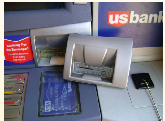
These are 2 examples of skimming devices placed over top of the actual card readers.
