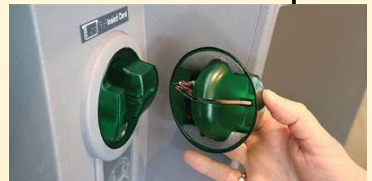
These are 2 examples of skimming devices placed over top of the actual card readers.
